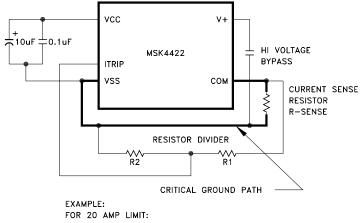
FOR 20 AMP LIMIT: R-SENSE = 0.050 OHMS R-SENSE VOLT = 1 VOLT R1 = 51.5 OHMS R2 = 48.5 OHMS
