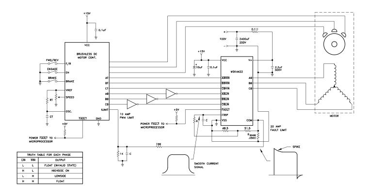
The MSK 4422 is designed to be used with a +100 volt high voltage bus, +15 volt low power bus and +5 volt logic signals. Proper derating should be applied when designing the MSK 4422 into a system. High frequency layout techniques with ground planes on a printed circuit board is the only method that should be used for circuit construction. This will prevent pulse jitter caused by excessive noise pickup on the current sense signal or the error amp signal.
